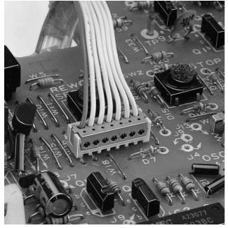
Measuring 2.0mm (.079") in pitch, only 5.0mm (.197") in mounting height, and 4.8mm (.189") in thickness, the DR connector is a compact insulation displacement connector developed to meet the needs for miniaturization of electronic equipment, including VCRs, cameras and car stereo systems.
