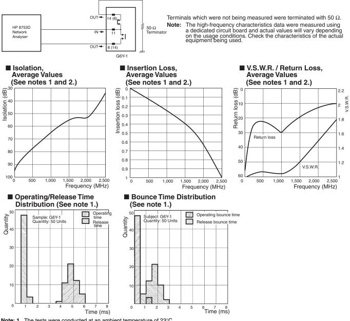
Note: 1. The tests were conducted at an ambient temperature of 23°C.
