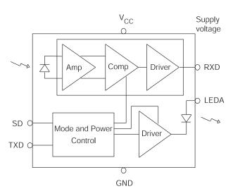
Figure 1. Slim SIR Transceiver Block Diagram
