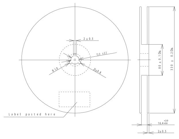
Figure 9. ZHX1810 Reel Dimensions (Unit: mm)
