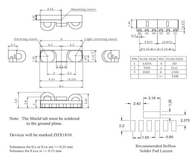
Figure 7. ZHX1810 Mechanical Drawing
