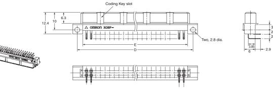
XC5F DIP terminal cross-section view
