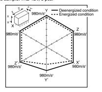
8-(2). Malfunctional shock (latching) Tested sample: TN2-L2-12V, 6 pcs.
