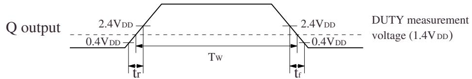
**Output duty cycle (CMOS)**
