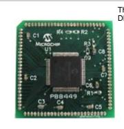
This is a 100-pin PIC24FJ256GA110 MCU sample for use with the Explorer 16 Development Board (DM240001 or DM240002).
