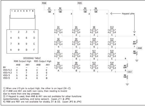
Figure 4-1: Keypad Hook-up Schematic
