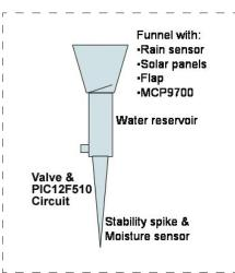
The Rose Protector: submitted by Maarten Hoffman (USA). This device protects roses by providing adequate water based on moisture and temperature using Microchip's PIC12F510 and MCP9700 devices.
