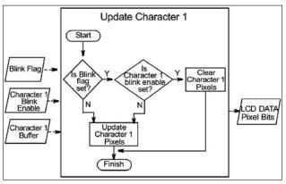
Fortunately, blinking is quite easy to implement. There are many ways to implement a blinking effect in software. Any regular event can be used to update a blink period counter. A blink flag can be toggled each time the blink period elapses. Each character or display element that you want to blink can be assigned a corresponding blink enable flag. The flowchart for updating the display would look as pictured in **Figure 3-2**.
