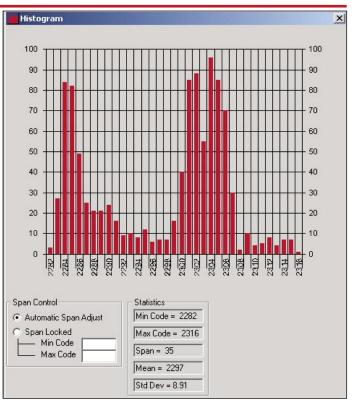
Figure 1: This histogram plot shows data from an ADC that is bimodal. It is difficult, if not impossible, to apply digital filtering to this data to recover a digital code that actually represents the input analog voltage accurately.
