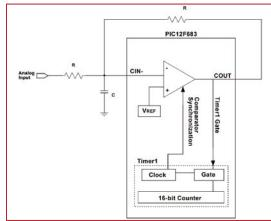
Figure 2: Delta-Sigma Converter Using the PIC12F683
