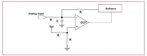
Figure 1: Delta-Sigma Converter Using a Standard Microcontroller
