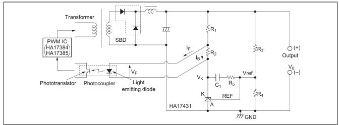
Figure 2 Typical Shunt Regulator/Error Amplifier
