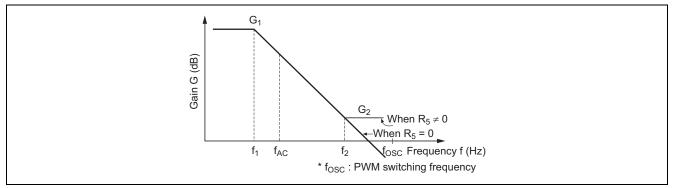
Figure 3 HA17431 Error Amplification Characteristic
