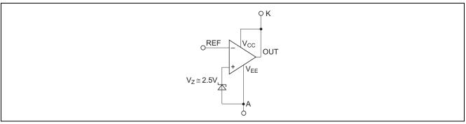
Figure 1 Operation Diagram
