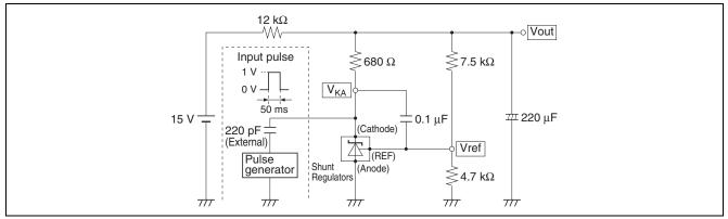
Figure 1 Noise Response Characteristics Measurement Circuit
