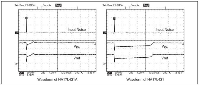
Figure 2 Noise Recovery Characteristics
