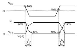
Fig. 6.2.2 Timing Chart of Switching Time
