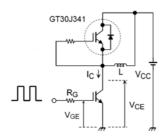
Fig. 6.2.1 Test Circuit of Switching Time
