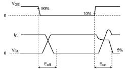
Fig. 6.2.3 Timing Chart of Switching Loss
