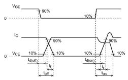
Fig. 6.2.2 Timing Chart of Switching Time
