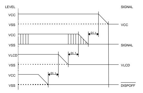
Please maintain the above sequence when turning on and off the power supply of the module.
