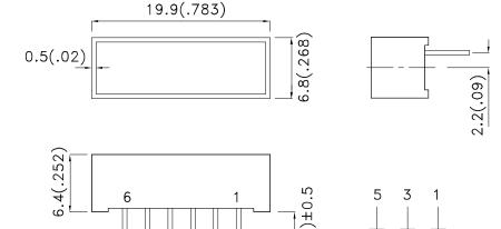
1.All dimensions are in millimeters (inches), Tolerance is  $\pm 0.25(0.01")$  unless otherwise noted. 2.Specifications are subject to change without notice.
