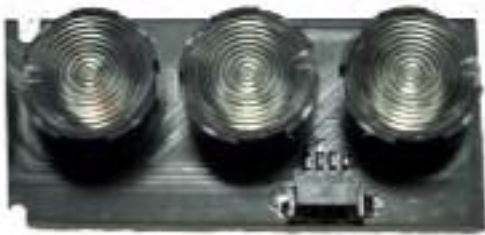
25 degree optics fitted and input connector detail
