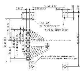
Recommended screw - M2.0 x length (thickness of PC board thickness of flange +2.0mm)
