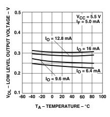
Figure 2. Low Level Output Voltage vs. Temperature.
