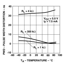
Figure 9. Pulse Width Distortion vs. Temperature.
