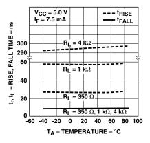
Figure 10. Rise and Fall Time vs. Temperature.
