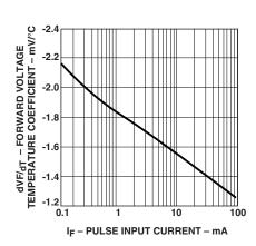
Figure 12. Temperature Coefficient for Forward Voltage vs. Input Current.
