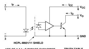
USE OF A 0.1  $\mu F$  BYPASS CAPACITOR MUST BE CONNECTED BETWEEN PINS 6 AND 4 (SEE NOTE 1).
