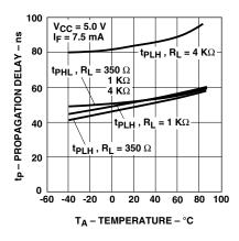
Figure 7. Propagation Delay vs. Temperature.
