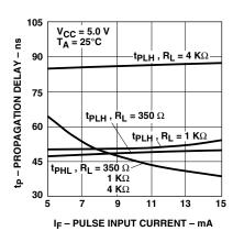
Figure 8. Propagation Delay vs. Pulse Input Current.
