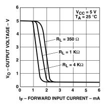
Figure 4. Output Voltage vs. Forward Input current.
