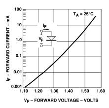
Figure 3. Input Diode Forward Characteristic.
