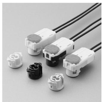
This connector for air-bag, conforming to ISO19072-4 standard configuration, has intelligent CPA, which allows locking the connector, incomplete mating detection and release of short-circuit at the same time.
